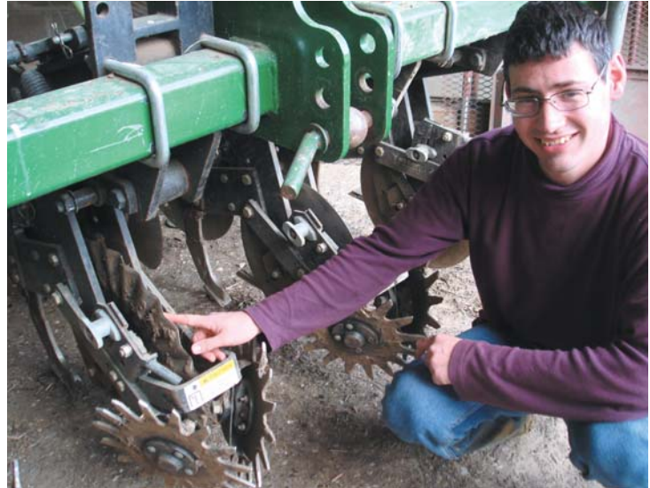
Nathan points to the star wheels for removing crop residue and fluted disc coultter for initial soil cultivation. "In the US farmers sometimes use a strip tilling machine that completes cultivation/drilling in one operation, particularly for maize on lighter soil. In the UK, particularly for sugar beet, we will more likely be looking at a machine that cultivates earlier in the year e.g. late autumn and then following with the drill in the spring when sugar beet is drilled," he said
